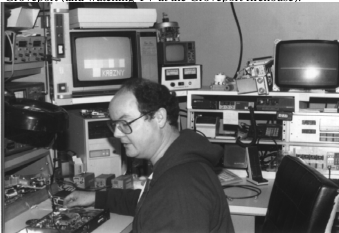
Tom working on his ATV transmitter exciter module
