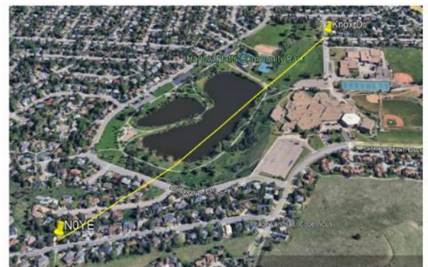
0.9 km clear line of sight RF path NOYE to KH6HTV
