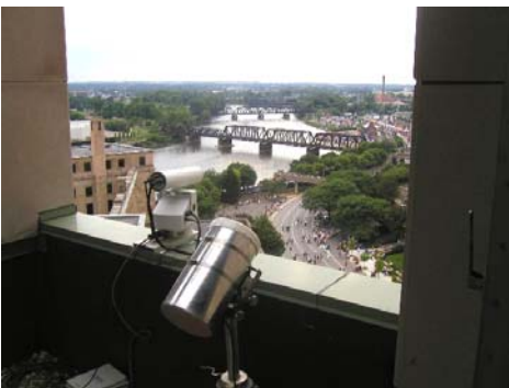
This shows the 1280MHz WU80 "Coffee Can" antenna pointing up to AEP building (shown below). It receives the AEP building roof camera.
