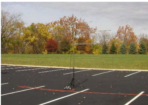
Here's a picture of the source antennas. The top one is a 42 element 2.4GHz loop yagi. Below that is the 439MHz yagi and on bottom is a small 1280MHz loop yagi.
