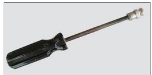
The completed tool aids in inserting or removing BNC jacks from a chassis without damaging the connector.
