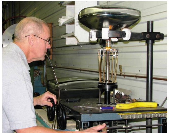
A new electron gun is sealed onto a small cathode ray tube. Avitt uses his breath to provide the small amount of air pressure necessary to keep the soft glass from collapsing.
