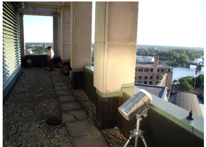
The above picture is "around the corner" from N8OCQ's location. Bob, W8RWR is in the background. The 1270MHz can antenna is receiving video from the AEP building roof.
