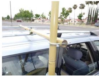
Figure 5 – Mast-brace attaches to roof-rack
