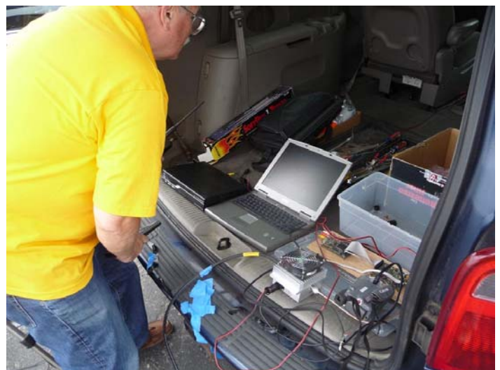
Figure 7 – Field DATV transmitting station in back of MiniVan (sniffer receiver display in center)
