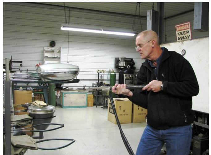
Scott Avitt applies the output coil from a large RF heater to a freshly rebuilt CRT. The heat produced will "fire" the tube's getter, depositing a silvery chemical compound on the neck that traps any gases or water vapor remaining after the tube has been sealed off from the vacuum pumps.
