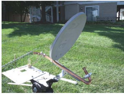
Here are pictures of the various 10 GHz portable rigs intended for "mountain top" operation. All are constructed in a way as to optimize a speedy set-up and for portability. Notice the unique feed arrangement of the one in the center. He chose to plumb the signal in copper pipe around to the back of the dish where the LNB is located. There were a number of people discussing this saying there could be serious phase problems. I didn't know what they were referring to but didn't want to appear dumb in company of the "experts".
