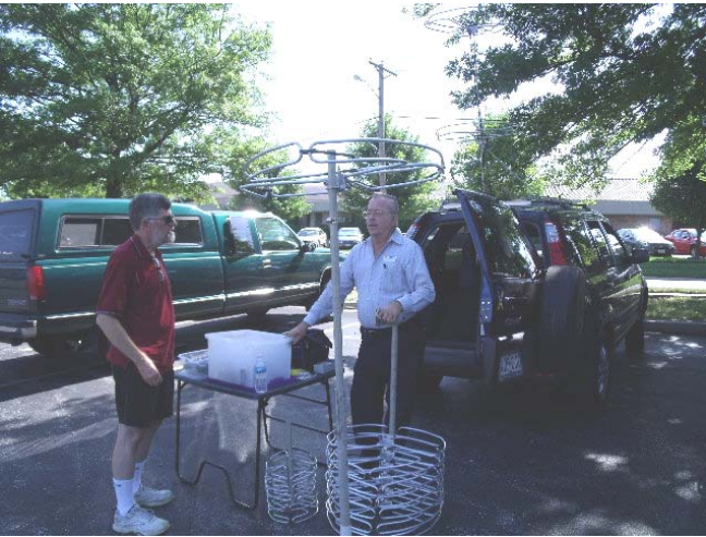
Here's a guy selling his version of the "Halo" antenna. He claims it works on both 144 & 220 MHz. I believe the price was $75. A smaller 440 MHz version is below the table.
