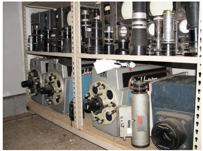
These RCA TK-60 cameras along with lenses, power supplies and monitors await full restoration. Pharis has enough vintage video gear to supply the studio needs of a large 1950's television network operation.
