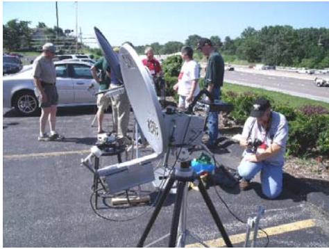
Here are pictures of the various 10 GHz portable rigs intended for "mountain top" operation. All are constructed in a way as to optimize a speedy set-up and for portability. Notice the unique feed arrangement of the one in the center. He chose to plumb the signal in copper pipe around to the back of the dish where the LNB is located. There were a number of people discussing this saying there could be serious phase problems. I didn't know what they were referring to but didn't want to appear dumb in company of the "experts".
