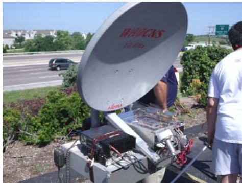
Here are pictures of the various 10 GHz portable rigs intended for "mountain top" operation. All are constructed in a way as to optimize a speedy set-up and for portability. Notice the unique feed arrangement of the one in the center. He chose to plumb the signal in copper pipe around to the back of the dish where the LNB is located. There were a number of people discussing this saying there could be serious phase problems. I didn't know what they were referring to but didn't want to appear dumb in company of the "experts".
