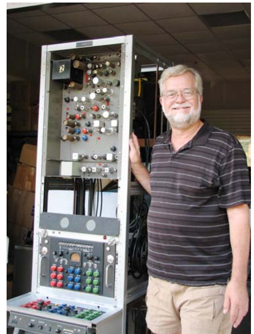
This recently acquired CCU and "Colorplexor" is the missing link for restoring to operation one of Pharis' RCA TK-41 three IO color cameras.
