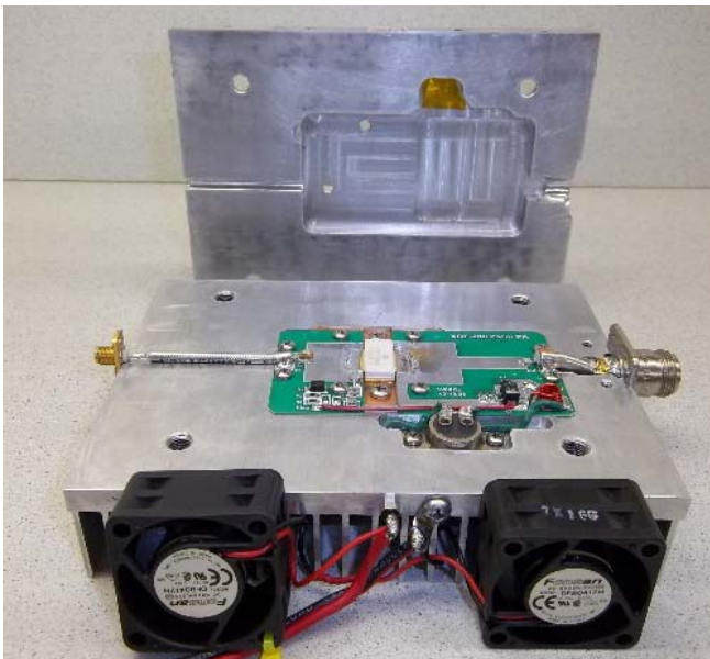
Here is an internal view with the aluminum blocks separated. The cover was milled out to fit the amp parts when put together.
