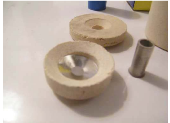
Figure III.2: The concave steel disc had dislocated, but was not a problem.
