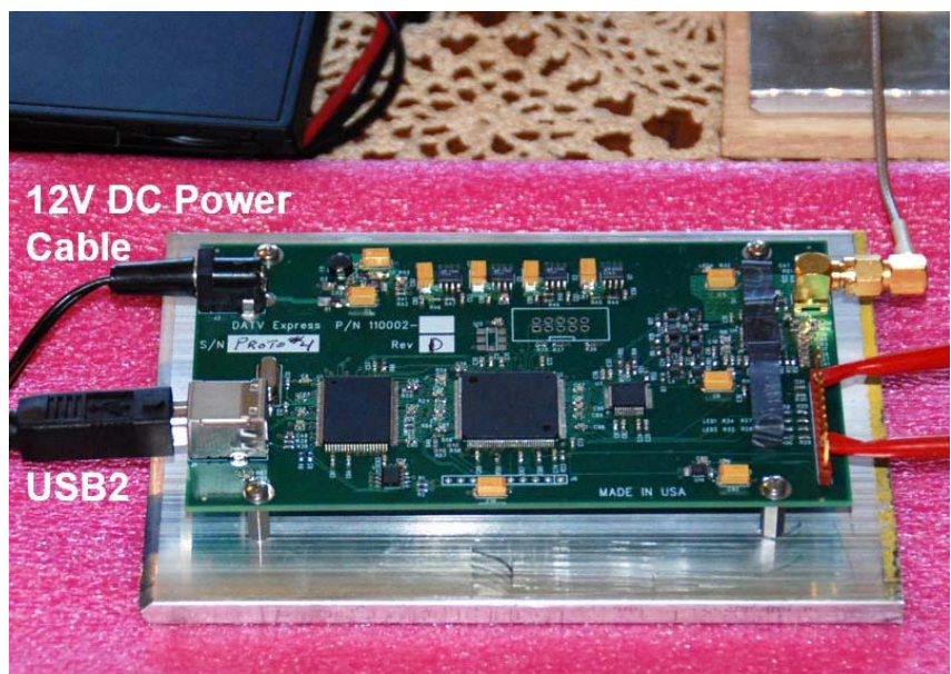
Figure 2 – The DATV-Express exciter hardware board is fitted with an aluminum plate as a heat-spreader.
