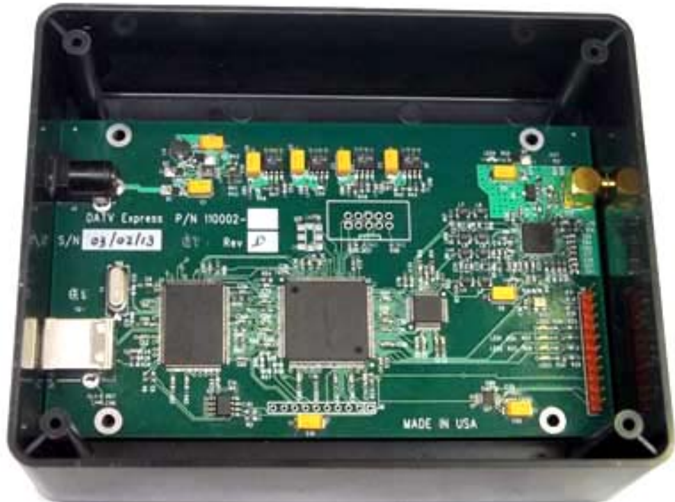
Fig 4 – the DATV-Express exciter board is a single printed circuit board mounted in a plastic project box.
