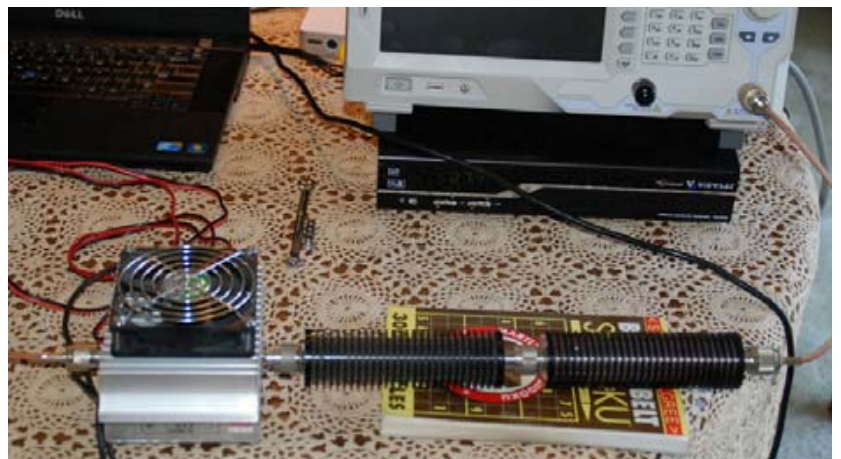
Figure 7 – The Down East RF Power Amp is connected to the Spectrum Analyzer through an external 40 dB of attenuation.
