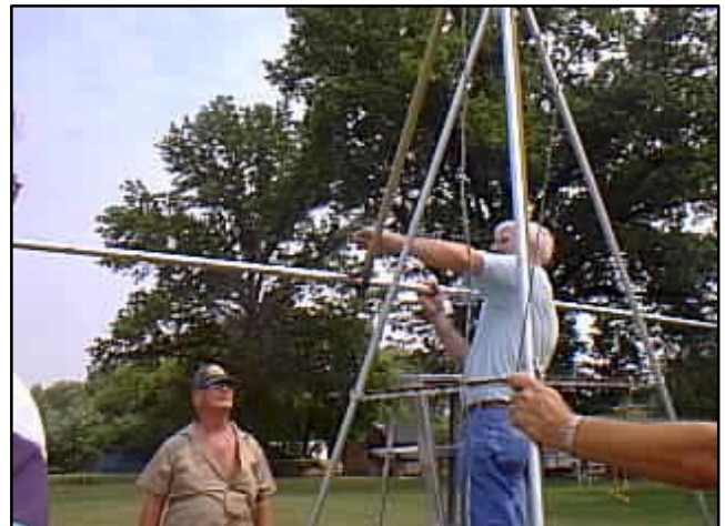
WA8RMC clamping another test antenna to the test jig
